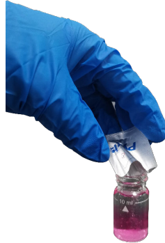
Figure 18. Add DPD powder to sample
