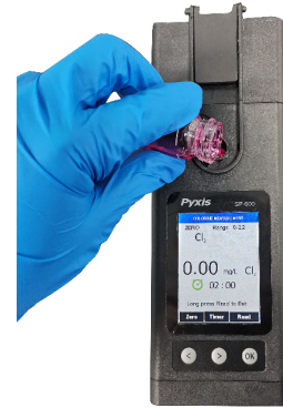
Figure 19. Fill sample cell with developed sample
