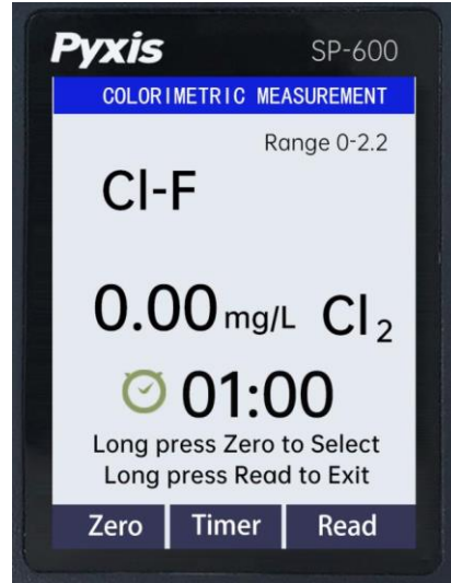
Figure 2. Zero sample before reagent addition
