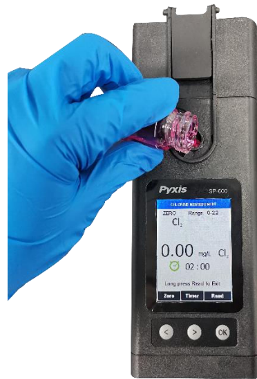
Figure 4. Transfer the developed sample to sample cell
